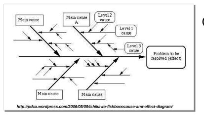
The Ishikawa diagram (also known as a Fishbone diagram) is a graphical method for finding the most likely causes for an undesired effect.
